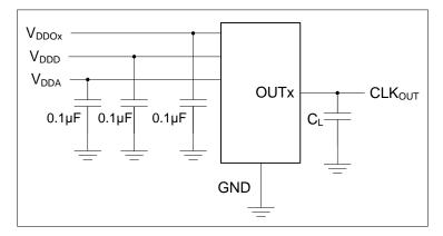
**Test Circuits and Loads for Outputs**
