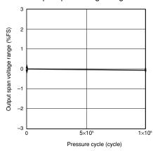
Even after testing for 1 million times, the variations in the offset voltage and output span voltage are minimal.
