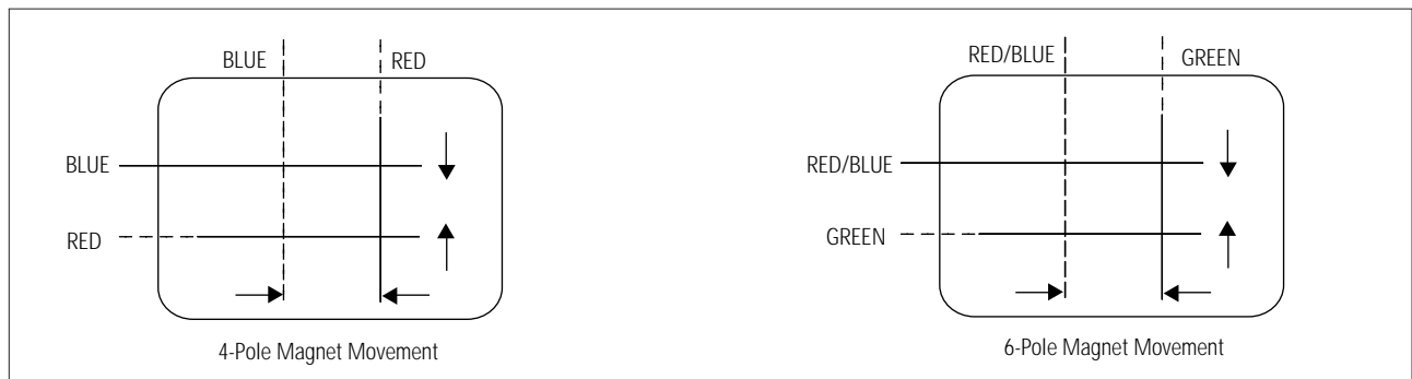
Fig. 4-5 Center Convergence Adjustment
