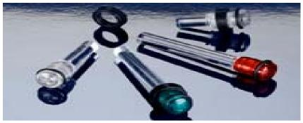
This lens and Litepipe® unit was developed to provide moisture sealing and dust control for display panels when the LED is attached to a circuit board. The LSS Series is designed for use with surface mount LEDs as well as standard thru-hole LEDs, horizontally or vertically circuit board mounted.
