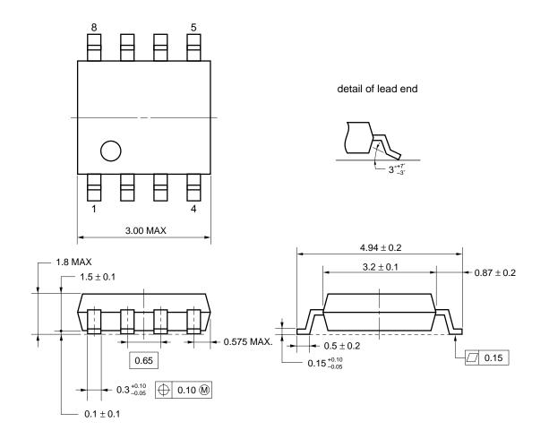
**NOTE** Each lead centerline is located within 0.10 mm of its true position (T.P.) at maximum material condition.
