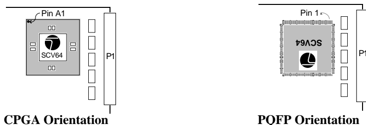
Figure E.1 : Orientation of the SCV64 (CPGA and PQFP) to Minimize Distance to the Connector
