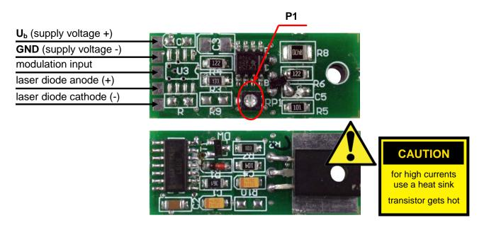
P1: trim pot for laser diode current adjustment
