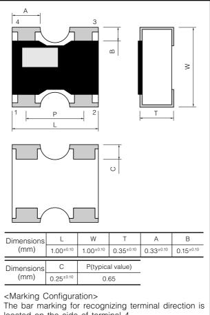
The bar marking for recognizing terminal direction is located on the side of terminal 4.
