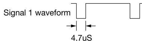
\*2 Measuring horizontal sync signal pull-in range for NTSC
