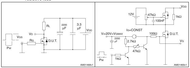
Figure 4. Test circuit for inductive load switching and diode recovery times
