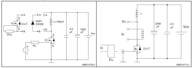
Figure 6. Unclamped inductive waveform
