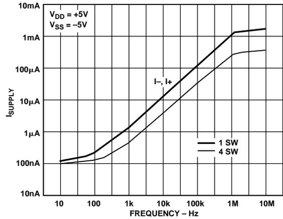
Figure 4. Supply Current vs. Input Switching Frequency
