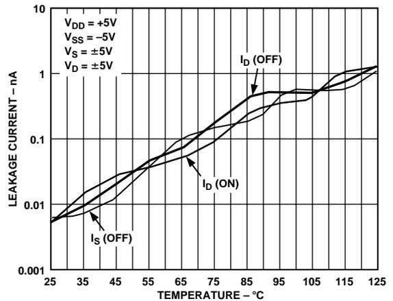
Figure 5. Leakage Currents as a Function of Temperature
