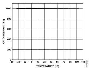
Figure 24. OV Threshold vs. Temperature
