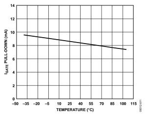
Figure 11. I<sub>GATE</sub> Pull-Down vs. Temperature
