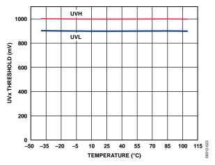
Figure 23. UVx Threshold vs. Temperature
