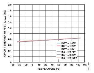
Figure 29. Circuit Breaker Offset vs. Temperature, ADM1075-1
