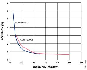
Figure 39. Worst-Case Current Sense Power Monitor Error vs. Current Sense  $Voltage(V_{SENSE})$
