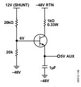
Figure 55. Powering iCoupler from -48 V Supply
