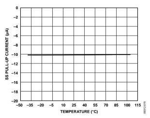
Figure 15. SS Pull-Up Current vs. Temperature
