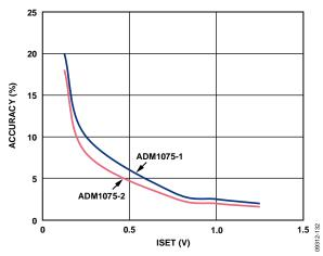
Figure 33. Worst-Case Hot Swap V<sub>SENSE</sub> Accuracy vs. ISET
