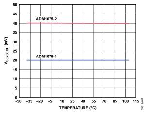
Figure 31.  $V_{SENSECL}$  vs. Temperature, ISET = 1.65 V
