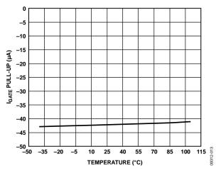
Figure 13. IGATE Pull-Up vs. Temperature
