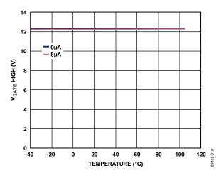
Figure 10. V<sub>GATE</sub> High vs. Temperature
