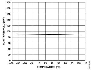
Figure 20. PLIM Threshold vs. Temperature
