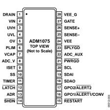
Figure 3. TSSOP Pin Configuration
