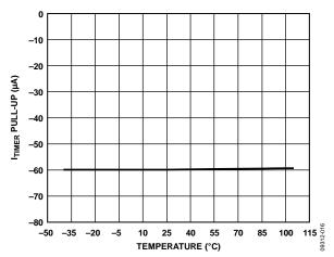
Figure 16. ITIMER Pull-Up vs. Temperature
