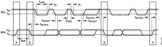
Figure 2. Serial Bus Timing Diagram
