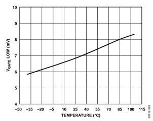
Figure 9.  $V_{GATE}$  Low vs. Temperature ( $I_{GATE} = 100 \mu A$ )
