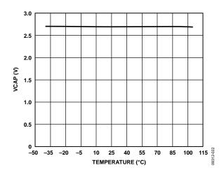
Figure 22. VCAP vs. Temperature ( $I_{VCAP} = 100 \mu A$ )
