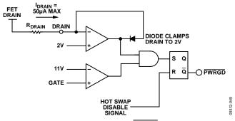
Figure 53. Generation of PWRGD Signal
