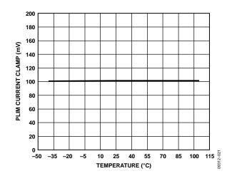
Figure 21. PLIM Current Clamp vs. Temperature
