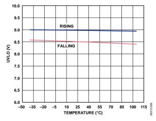
Figure 8. UVLO vs. Temperature
