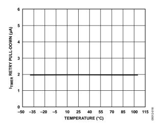
Figure 18. ITIMER Retry Pull-Down vs. Temperature
