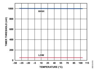
Figure 19. TIMER Threshold vs. Temperature
