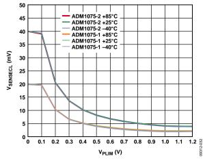
Figure 32. V<sub>SENSECL</sub> vs. PLIM
