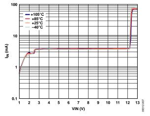
Figure 7. IIN vs. VIN
