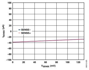
Figure 25. Isense vs. Vsense
