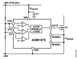
Figure 52. Undervoltage and Overvoltage Supply Monitoring
