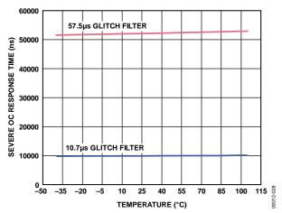
Figure 28. Severe OC Response vs. Temperature
