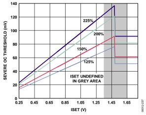
Figure 38. Severe OC Threshold vs. ISET, ADM1075-2
