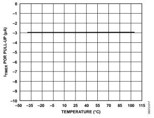
Figure 17. ITIMER POR Pull-Up vs. Temperature
