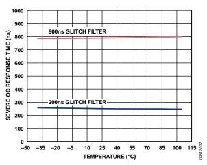
Figure 27. Severe OC Response vs. Temperature
