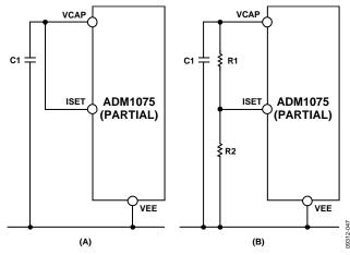
Figure 48. (a) Fixed 20 mV/40 mV Current Sense Limit (b) Adjustable 15 mV to 50 mV Current Sense Limit
