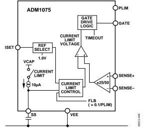
Figure 46. Current Limit Reference Selection
