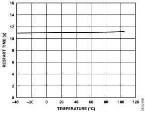
Figure 26. Restart Time vs. Temperature
