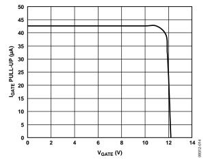
Figure 14. IGATE Pull-Up vs. VGATE
