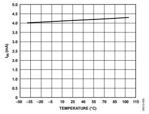
Figure 5. I<sub>IN</sub> vs. Temperature
