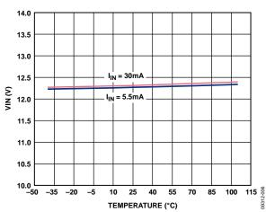
Figure 6. VIN vs. Temperature
