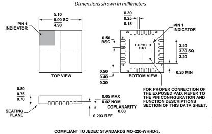
Figure 66. 28-Lead Lead Frame Chip Scale Package [LFCSP\_WQ]
