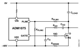
Figure 51. Required Extra Components
