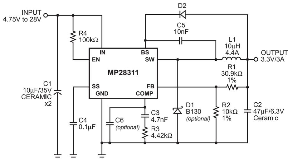
**Figure 4—MP28311 with 3.3V Output, 47µF/6.3V Ceramic Output Capacitor**
