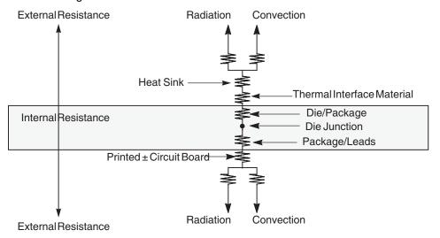
Note the internal versus external package resistance.
