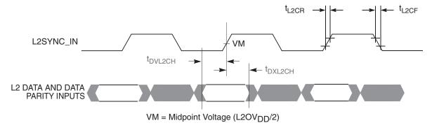
Figure 16 shows the L2 bus output timing diagrams for the PC755.
