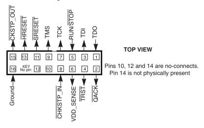
There is no standardized way to number the COP header shown in Figure 24; consequently, many different pin numbers have been observed from emulator vendors. Some are numbered top-to-bottom then left-to-right, while others use left-to-right then top-to-bottom, while still others number the pins counter clockwise from pin one (as with an IC). Regardless of the numbering, the signal placement recommended in Figure 24 is common to all known emulators.
