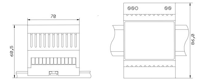
Case material is for the top cover (Lexan), lower case (Noryl) . Class UL94V0 Top cover includes ventilating louvers for cooling by air convection
