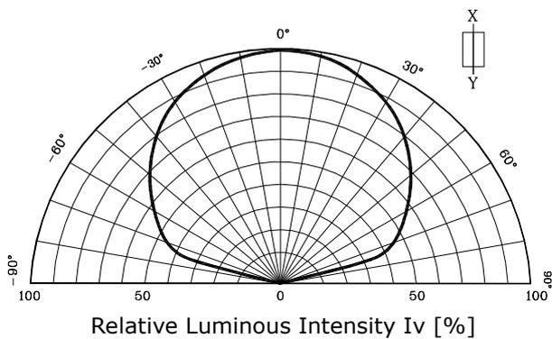
Fig. 5-2 Radiation Diagram(Y)
