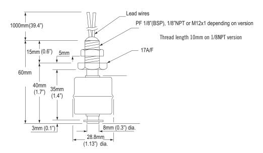
The SSF22 series is a compact vertical internally mounted device. Mounting is in the top or bottom of the tank from the inside, so requires access to the inside of the tank.
