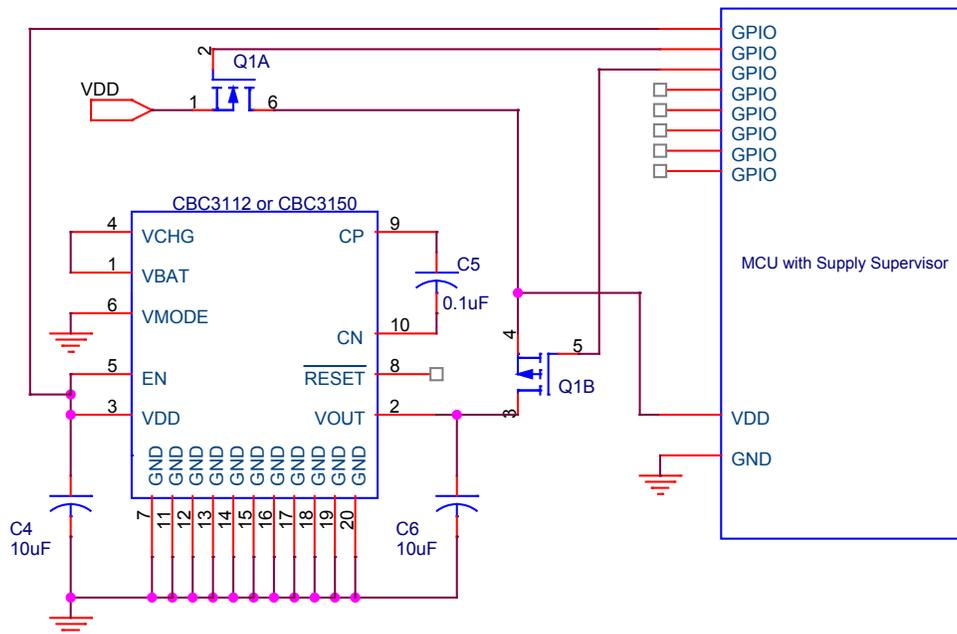
Figure 1. Typical Application Circuit Using the EnerChip CC and Microcontroller for Ultra Low Power Operation.
