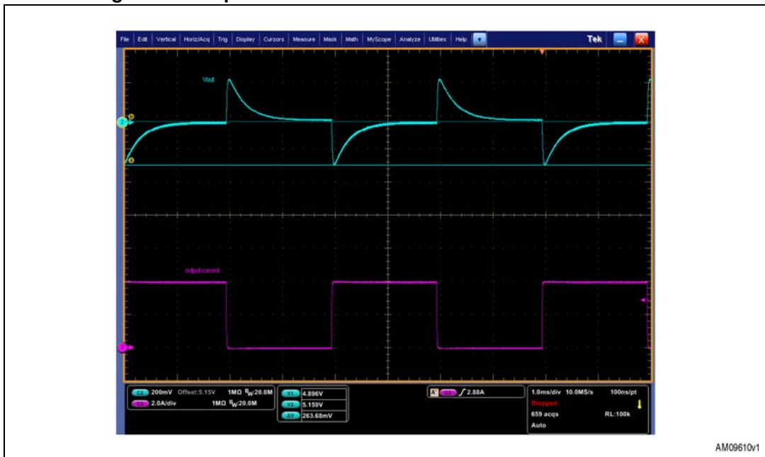
Figure 27. Response of the converter to a 0 A - 4 A load transient
