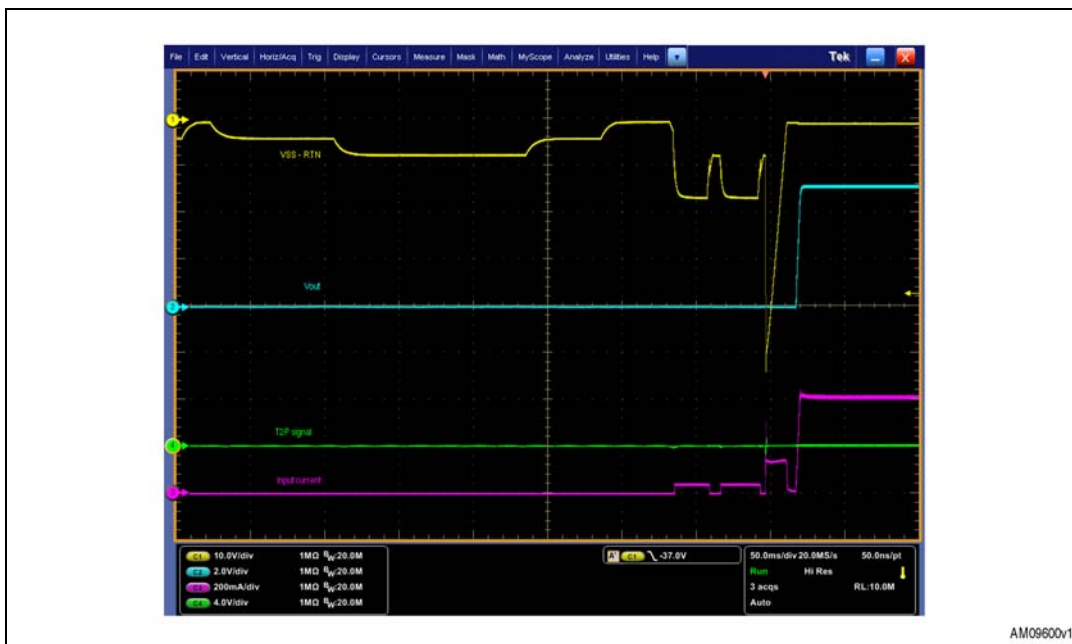
Figure 17. Startup from an IEEE 802.3at injector with 4 A load
