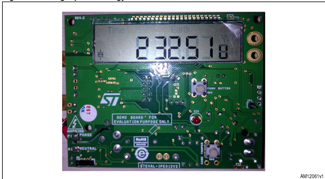
Figure 1. Single-phase energy meter solution based on STPM10 and STM8L152C6
