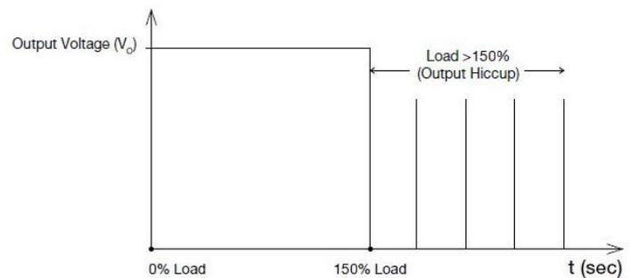
Additionally, if the  $I_o$  is  $<115\%$  but  $>100\%$  for a prolong period of time (depending on the load), the Over Temperature Protection (OTP) will be activated due to high temperature on critical components. The power supply will then go into hiccup mode until the fault is removed and the mains is reapplied.
