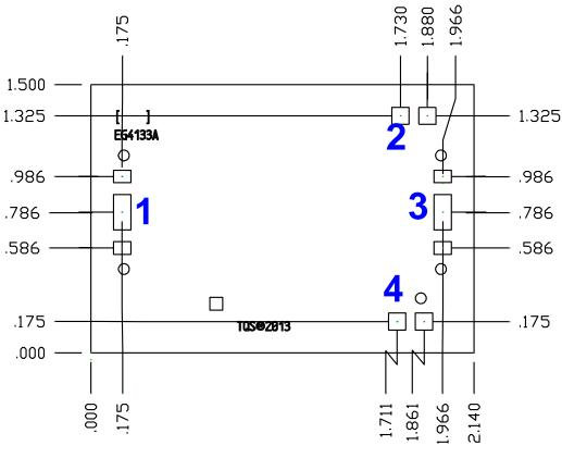
Unit: millimeters Thickness: 0.10 Die x, y size tolerance: +/- 0.050 Chip edge to bond pad dimensions are shown to center of pad Ground is backside of die
