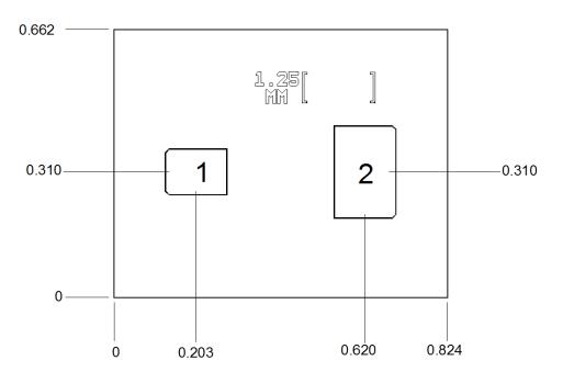
Units: millimeters Thickness: 0.100 Die x,y size tolerance: +/- 0.050
