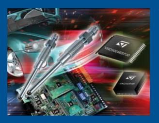
The VND5004B from **STMicroelectronics** is a dual-channel low  $R_{DS(ON)}$  device (4 m $\Omega$  per channel) in VIPower<sup>TM</sup> M0-5 technology.
