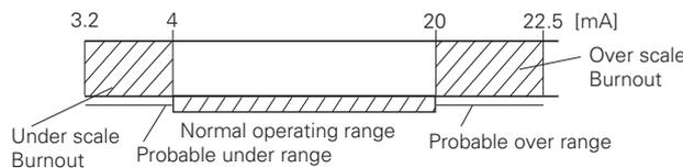
**Loop-check output:** Transmitter can be configured to provide constant signal 3.2mA through 22.5mA by HHC.
