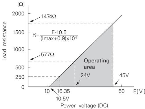
Note: For communication with HHC<sup>(1)</sup> (Model: FXW), min. of 250Ω required.
