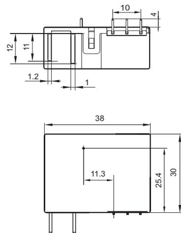
Remark: 1) In case of no tolerance shown in outline dimension: outline dimension  $\leq 1$ mm, tolerance should be  $\pm 0.2$ mm; outline dimension  $> 1$ mm and  $\leq 5$ mm, tolerance should be  $\pm 0.3$ mm; outline dimension  $> 5$ mm, tolerance should be  $\pm 0.4$ mm.
