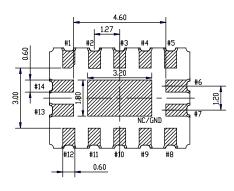
OE pin = "H" : Specified frequency output. OE pin = "L" : Output is high impedance #14 is connected to the cover.
