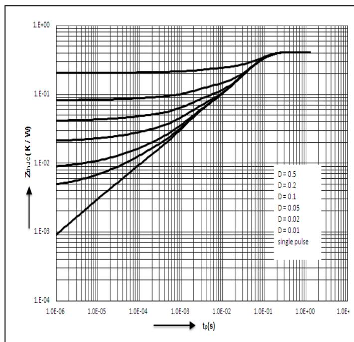
Figure 4. Maximum Effective Transient Thermal Impedance, Junction-to-Case
