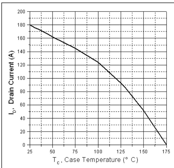
Figure 3. Maximum Drain Current Vs. Case Temperature
