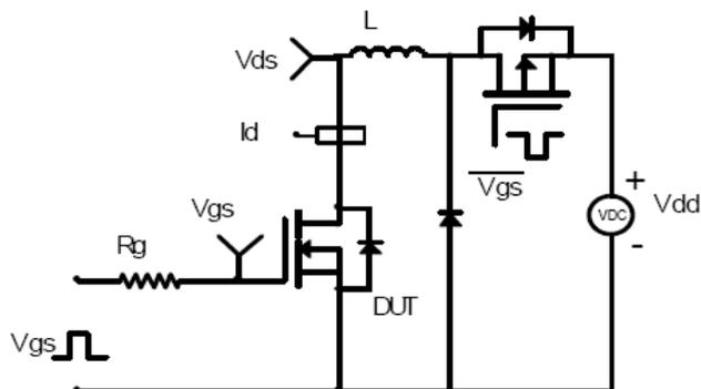
Gate charge test circuit:
