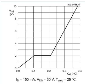
Fig. 15. Gate charge waveform definitions
