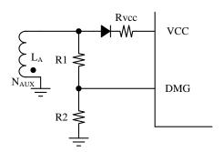
$$Vo_{OVP} = \frac{NSEC}{NAUX} \times VOVPS \times \frac{R_1 + R_2}{R_2}$$
