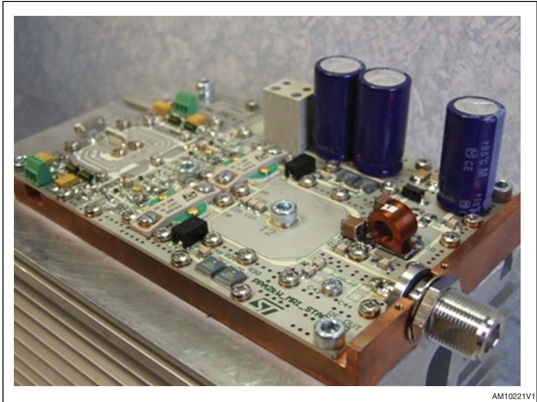
Figure 4. 2 kW MRI final assembled board
