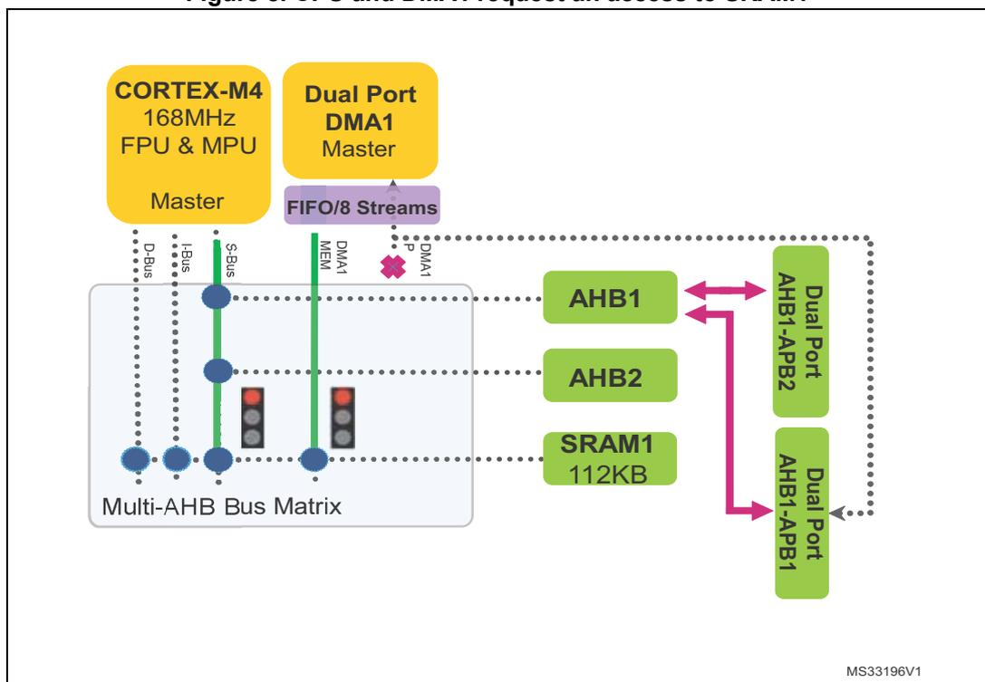
In case of bus access concurrency as in the above example, a bus matrix arbitration is required. The round-robin policy is then applied in order to solve the issue: if the last master which won the bus was the CPU, during the next access DMA1 wins the bus and accesses SRAM1 first. The CPU has then the rights to access SRAM1.
