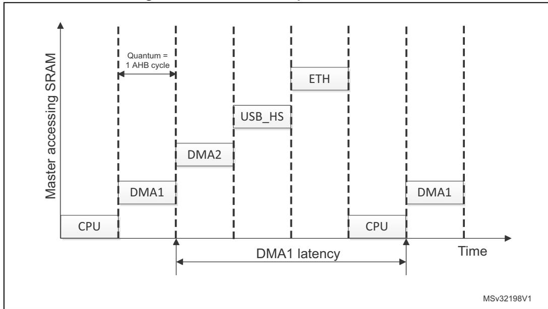
The latency associated to DMA1 to win the bus matrix again and access SRAM1 (for example) is equal to the execution time of all pending requests coming from the other masters.
