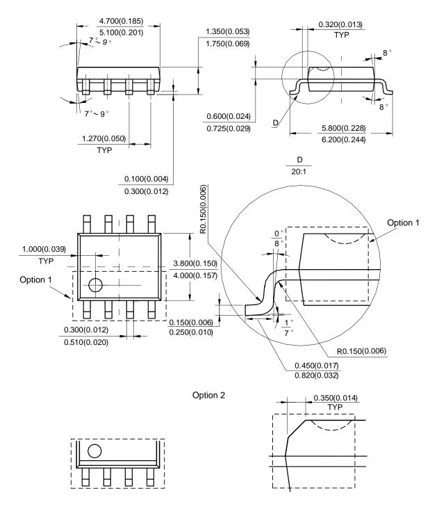
Note: Eject hole, oriented hole and mold mark is optional.
