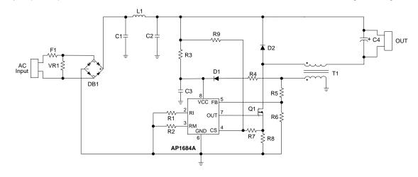
Figure 1. Typical BUCK Application Circuit
