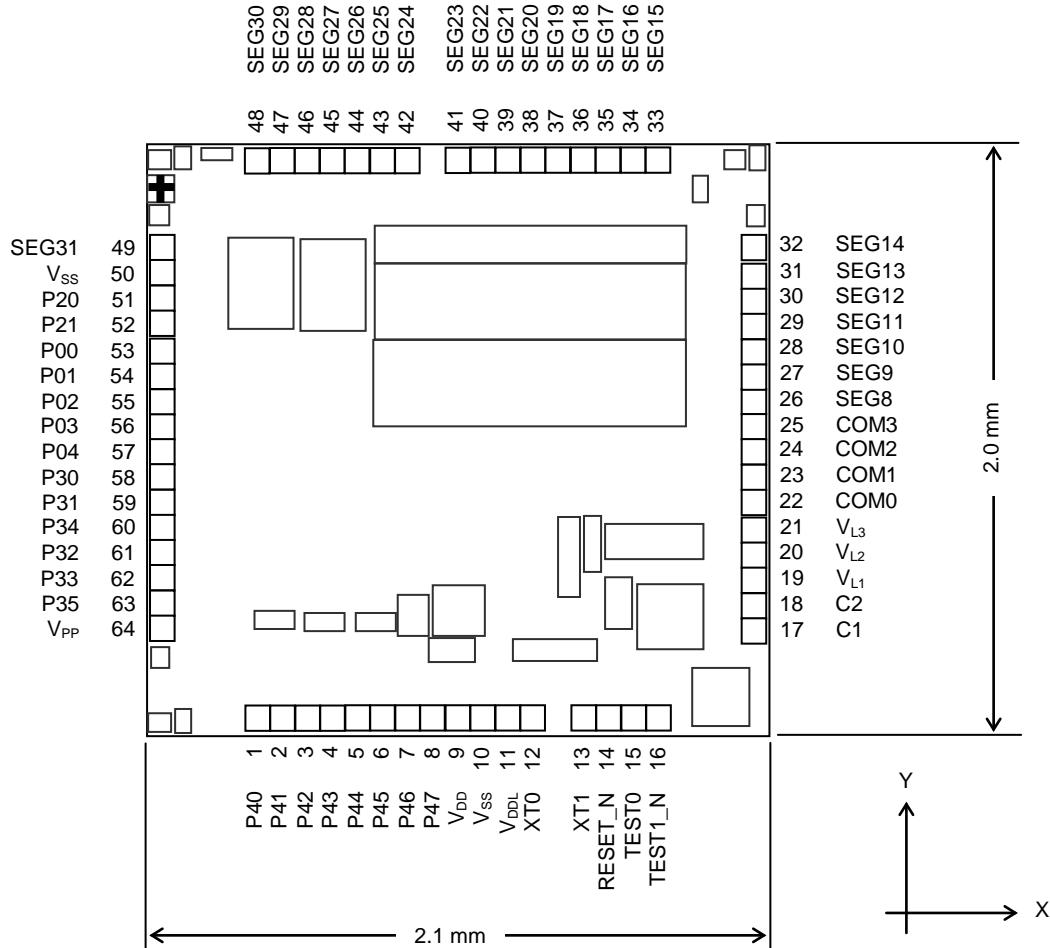
Note: The assignment of the pads P30 to P35 are not in order.
