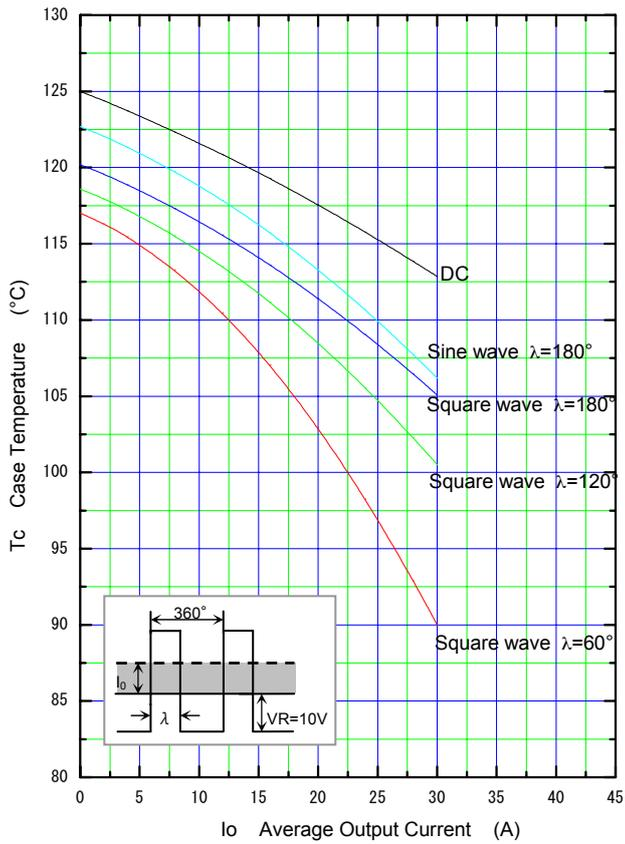
$\lambda$ : Conduction angle of forward current for each rectifier element
