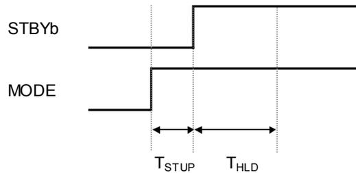
Figure 1: STBYb/MODE input timing
