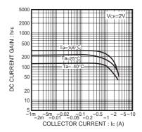
Fig.3 DC Current Gain vs. Collector Current
