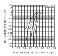
Fig.2 Grounded Emitter Propagation Characteristics
