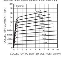
Fig.1 Grounded EmitterOutput Characteristics
