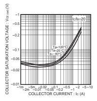
Fig.4 Collector-Emitter Saturation Voltage vs. Collector Current
