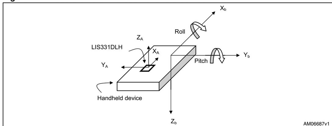
$X_b$ ,  $Y_b$  and  $Z_b$  are the handheld device body axes with a forward-right-down configuration.
