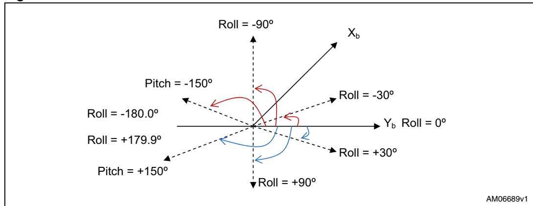
Assume  $A_x$ ,  $A_y$ ,  $A_z$  is the accelerometer raw measurement in the format of LSBs. [Table 2](#) shows the sign definition of the raw sensor data at 6 stationary positions with respect to the known Earth gravity vector. For example, in [Figure 1](#),  $X_b$  and  $Y_b$  are level and  $Z_b$  is pointing down. Therefore,  $A_x = A_y = 0$ ,  $A_z = +1 g$ .
