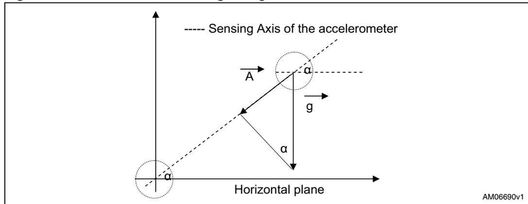
The accelerometer measures the projection of the gravity vector on the sensing axis. The amplitude of the sensed acceleration changes as the sin of the angle  $\alpha$  between the sensitive axis and the horizontal plane.
