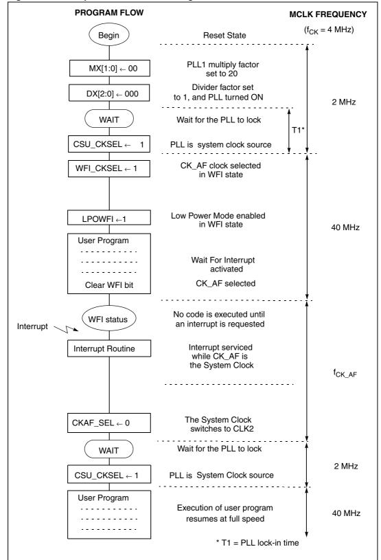
Figure 4. Example of LPWFI mode using CK\_AF
