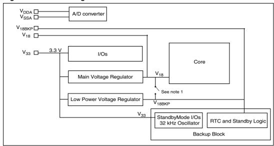
In normal operation, the switch connecting the V18 domain and the V18BKP domain is closed, it is opened only during STANDBY mode (refer to Section 4)
