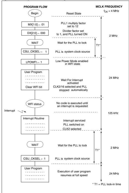
Figure 5. Example of LPWFI mode using CLK2/16
