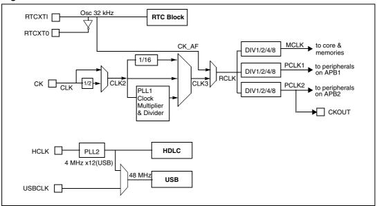
The source clock CLK is derived from an external oscillator, through the CK pin. This clock may be turned off during Low power modes. (refer to *Section 4*).
