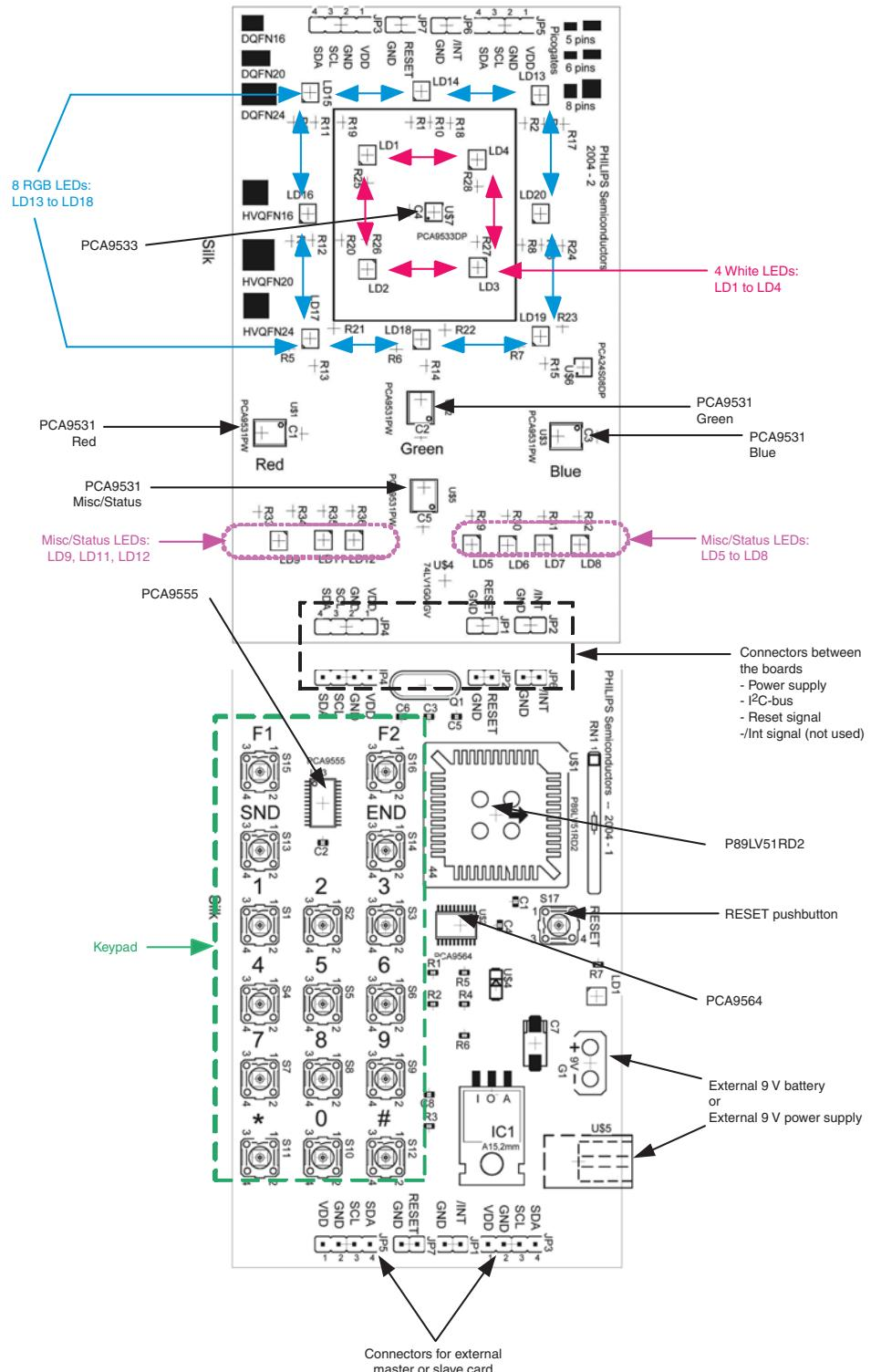
**Fig 4.** Schematic keypad control card
