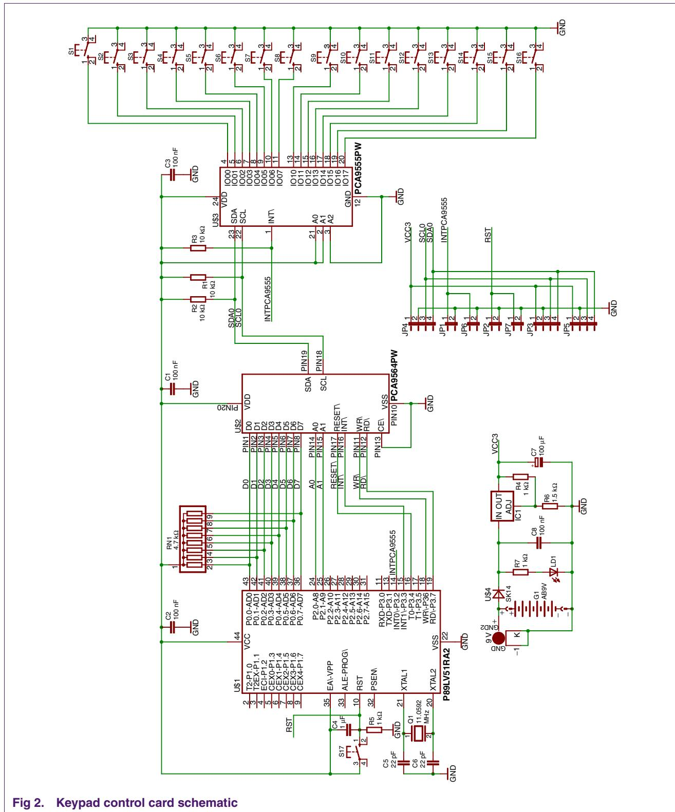
Fig 2. Keypad control card schematic
