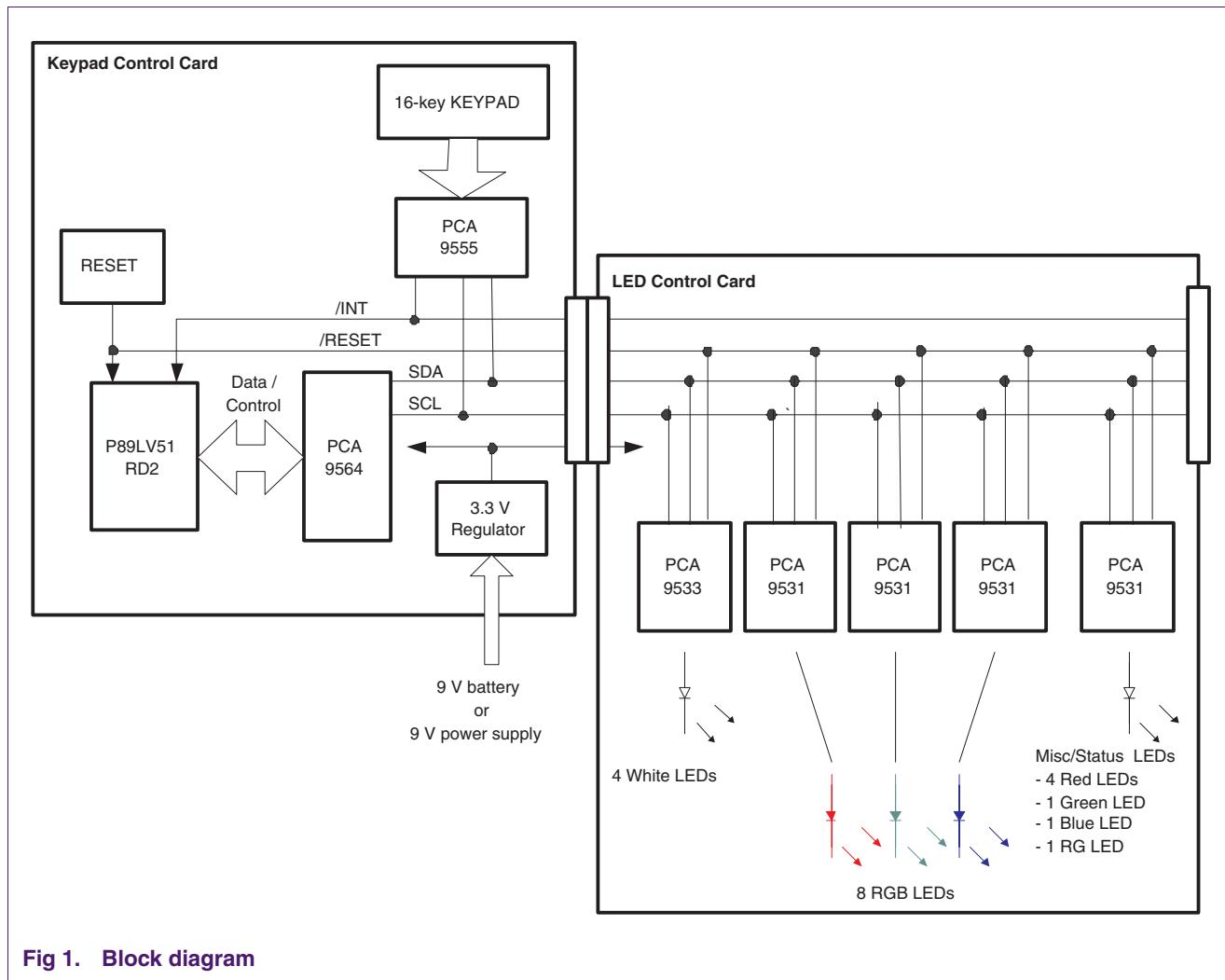
Fig 1. Block diagram
