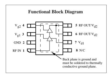
mum performance and flexibility. The CMM0336 is packaged in a low-cost, space efficient SO-8 power package that gives excellent electrical stability and thermal handling performance with a  $R_{\Theta}$  of less than 18° C/W. The part is designed to require minimal external circuitry for bias matching, simplifying design and keeping board space and cost to a minimum.
