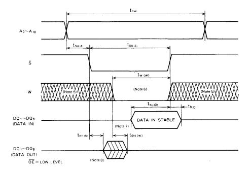
Note 4 Test conditions Input pulse level:  $0.4 \sim 2.4 \text{V}$  Input pulse risetime and fall time: 10ns Load: 1TTL,  $C_L = 100 \text{pF}$  Reference level: 1.5 V
