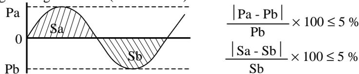
Pa: Supply voltage/current peak for positive, Pb: Supply voltage/current peak for negative
