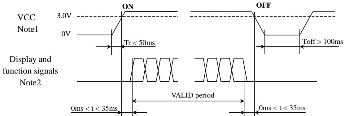
Note1: In terms of voltage variation (voltage drop) while VCC rising edge is below 3.0V, a protection circuit may work, and then this product may not work.
