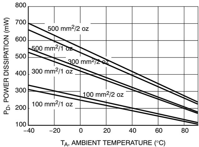
**Figure 6. Power Dissipation vs. Ambient Temperature @  $T_j = 150^\circ\text{C}$**
