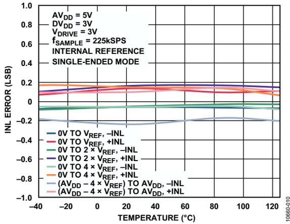
Figure 10. ADC INL vs. Temperature
