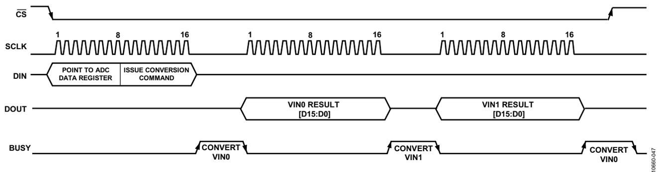
Figure 41. ADC Conversion Command (ADC Sequencer Used)
