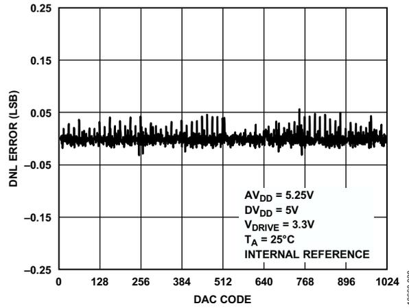
Figure 20. Typical DAC DNL vs. Output Code
