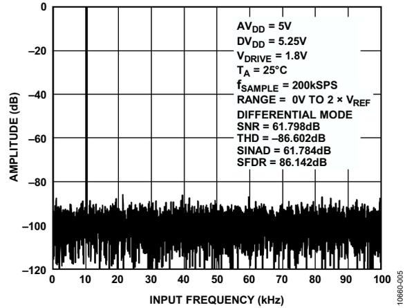
Figure 7. ADC FFT, 200 kSPS,  $f_{IN} = 10$  kHz, Differential Mode
