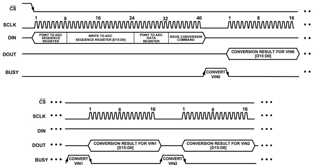
Figure 43. Example of Using the ADC Sequencer
