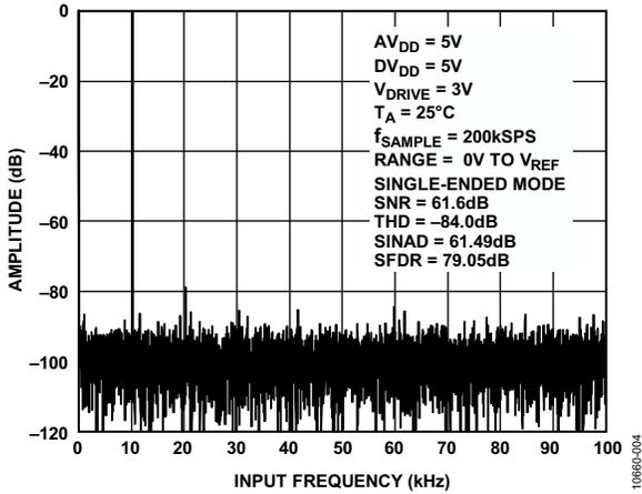
Figure 4. ADC FFT, 200 kSPS,  $f_{IN} = 10$  kHz, Single-Ended Mode
