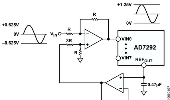
Figure 31. Interfacing to a Bipolar Input Signal
