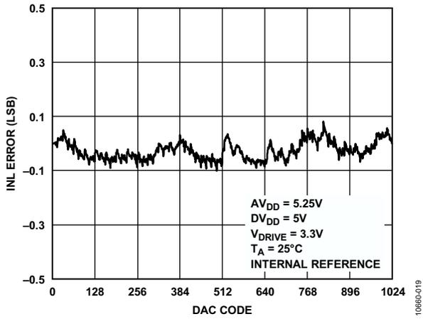
Figure 17. Typical DAC INL vs. Output Code
