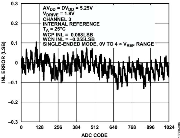
Figure 5. Typical ADC INL, Single-Ended Mode
