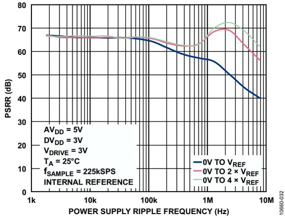
Figure 29. PSRR vs. Power Supply Ripple Frequency
