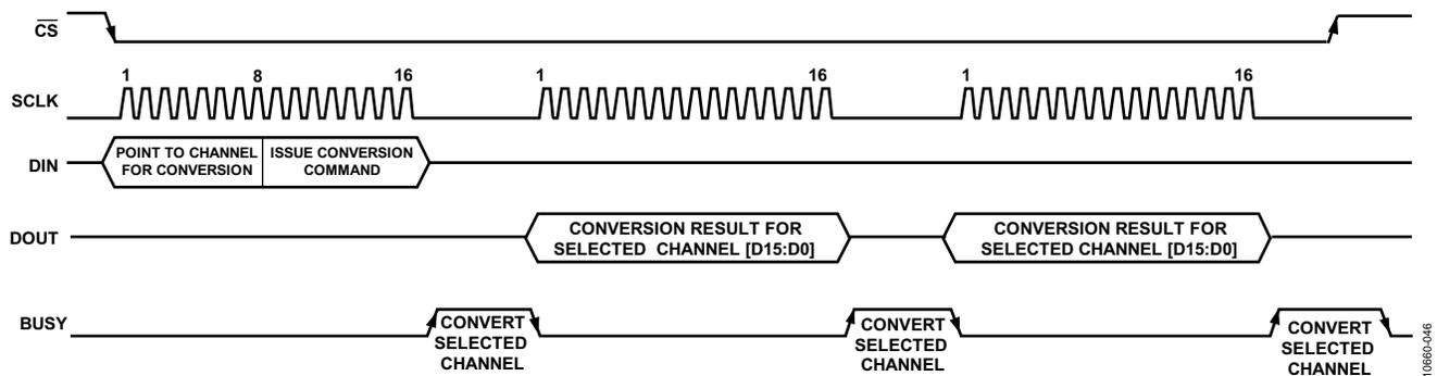
Figure 40. ADC Conversion Command (ADC Sequencer Not Used)
