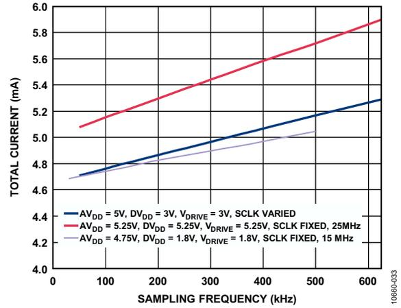
Figure 30. Total Supply Current vs. Throughput Rate
