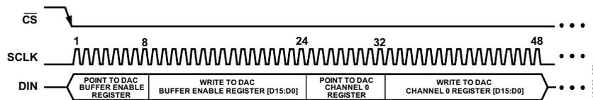
Figure 44. Setting the DAC Output Voltage Code
