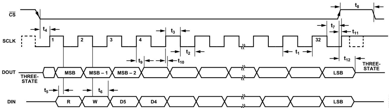
Figure 35. Serial Interface Timing Diagram
