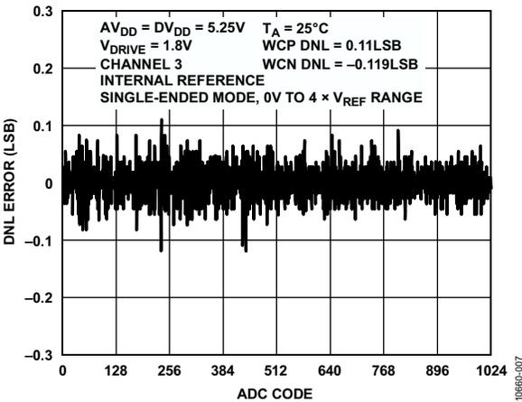
Figure 6. Typical ADC DNL, Single-Ended Mode
