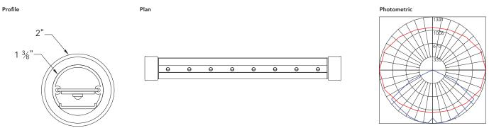
Maximum Candela = 1340.9 Located At Horizontal Angle = 0, Vertical Angle = 5 # 1 - Vertical Plane Through Horizontal Angle = 0, Vertical Angle = 5 # 2 - Horizontal Cone Through Vertical Angle (5) (Through Max. Cd.)
