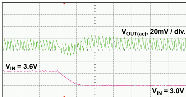
Figure 28. Line Transient, 600mV, 50mA Load
