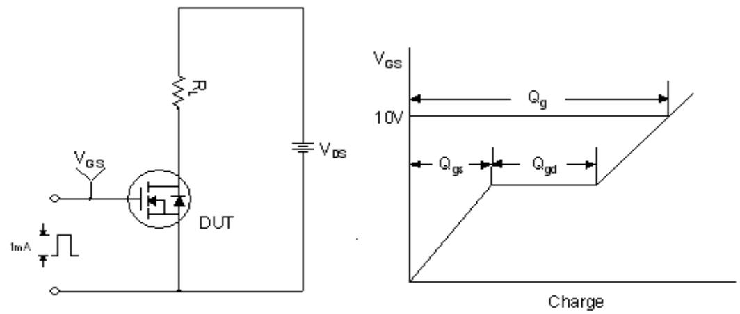
**Resistive Switching Test Circuit & Waveforms**
