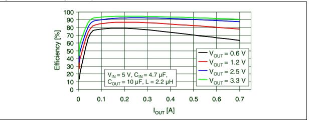
Figure 15. Efficiency vs. output voltage
