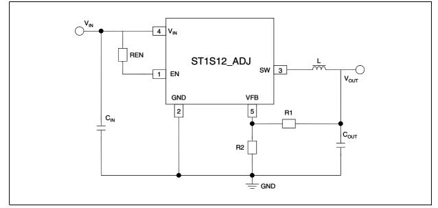
The R<sub>EN</sub> is used to pull up the EN pin to V<sub>IN</sub>. We suggest using a resistor with a value in the range of 500 k $\Omega$  to 1 M $\Omega$  in order to reduce current consumption.
