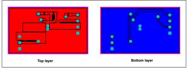
The board has one enable pin available which is located on the right side of the board. This pin can be used to supply the enable pin with a external voltage higher than 1.5 V to turn on or lower than 0.5 V to turn off the device.
