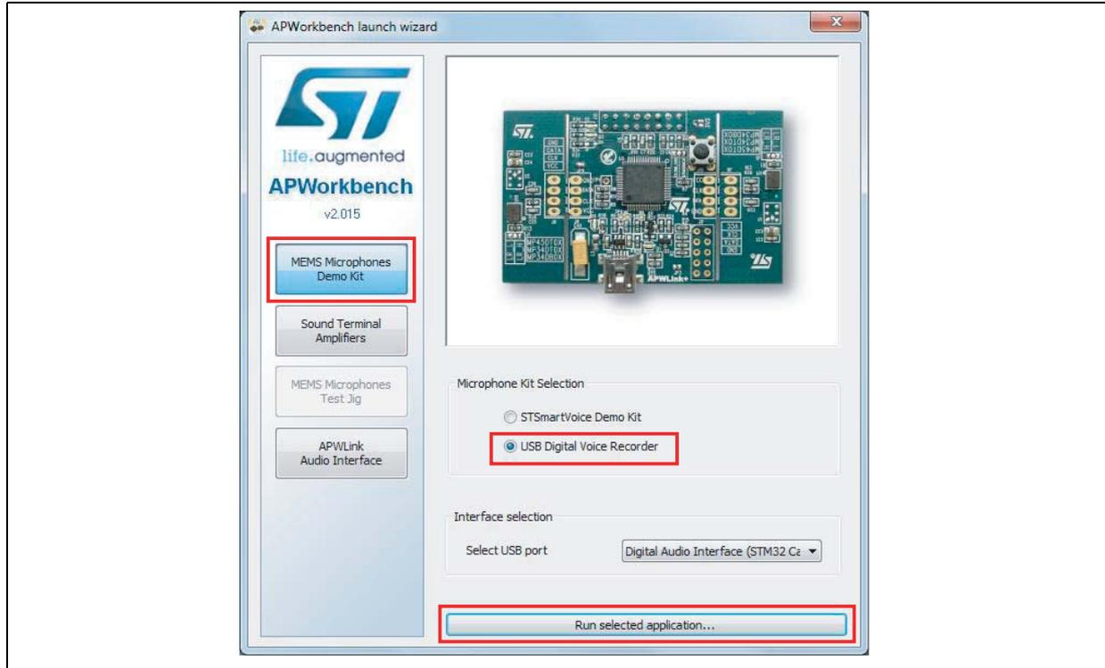
Once this selection has been run, a dedicated panel will appear. If the user wants to operate the board as a USB voice recorder, the tool shows the panel performing either FFT or scope monitoring. It is also possible to record the signal sensed by the microphones on the board.
